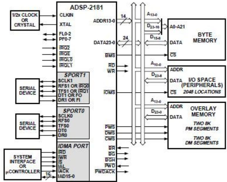
Figure 2. ADSP-2181 Basic System Configuration
