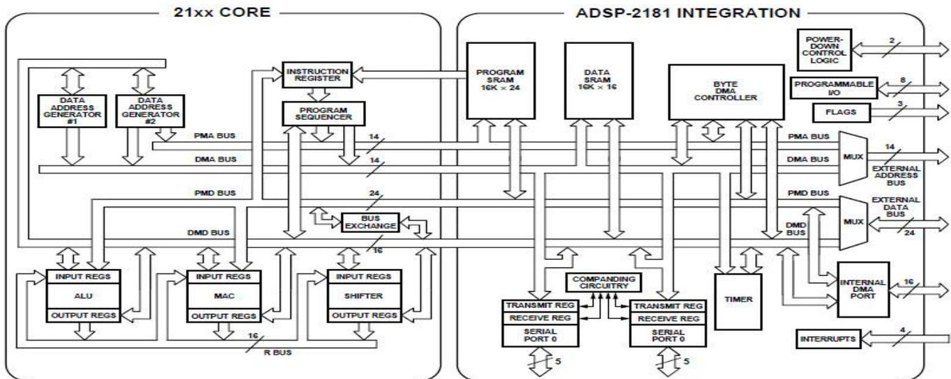
Figure 1. ADSP-2181 Block Diagram
